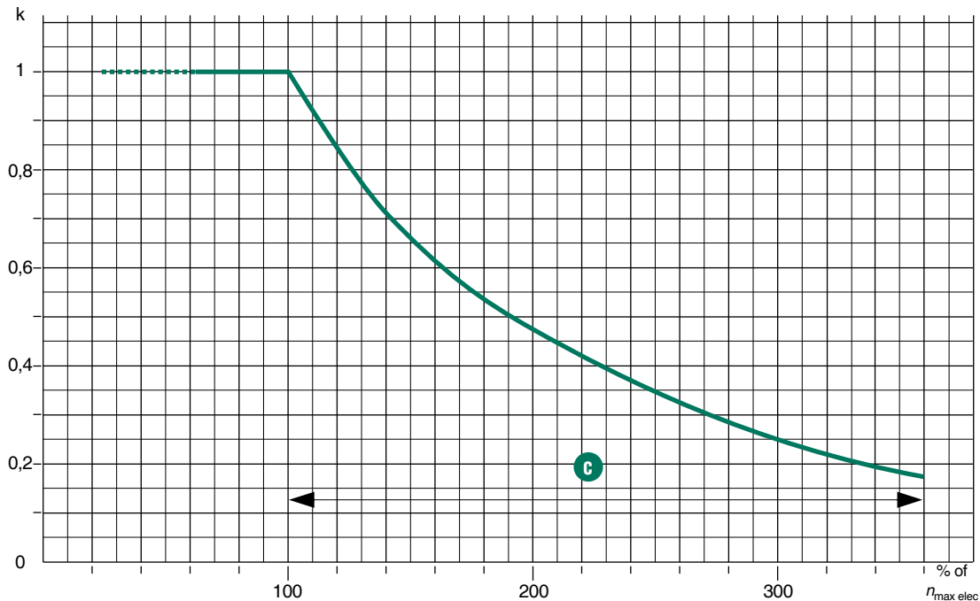
Curve 5. - Power correction coefficient k as a function of speed variation by field
